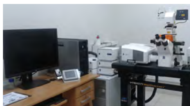
Confocal fluorescence microscope LSM 780 (Carl Zeiss) for multiple laser lines (405, 458, 488, 514, 543, 633 nm)
